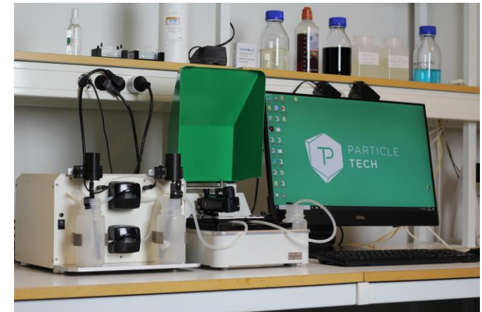
Sampling automatically pumped into flow cell
